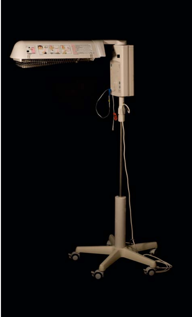
Figure 30.4 An infrared radiant warmer for infants.
