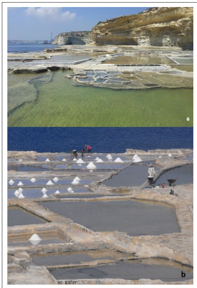
Figure 6. Shore platform at Delimara Point, with salinas belonging to the Mangion family: (a) The upper section of the salinas with evaporation basins and smaller premodern salinas in the foreground; (b) evaporation basins and crystallizers in the lower section of the platform during harvesting time.
