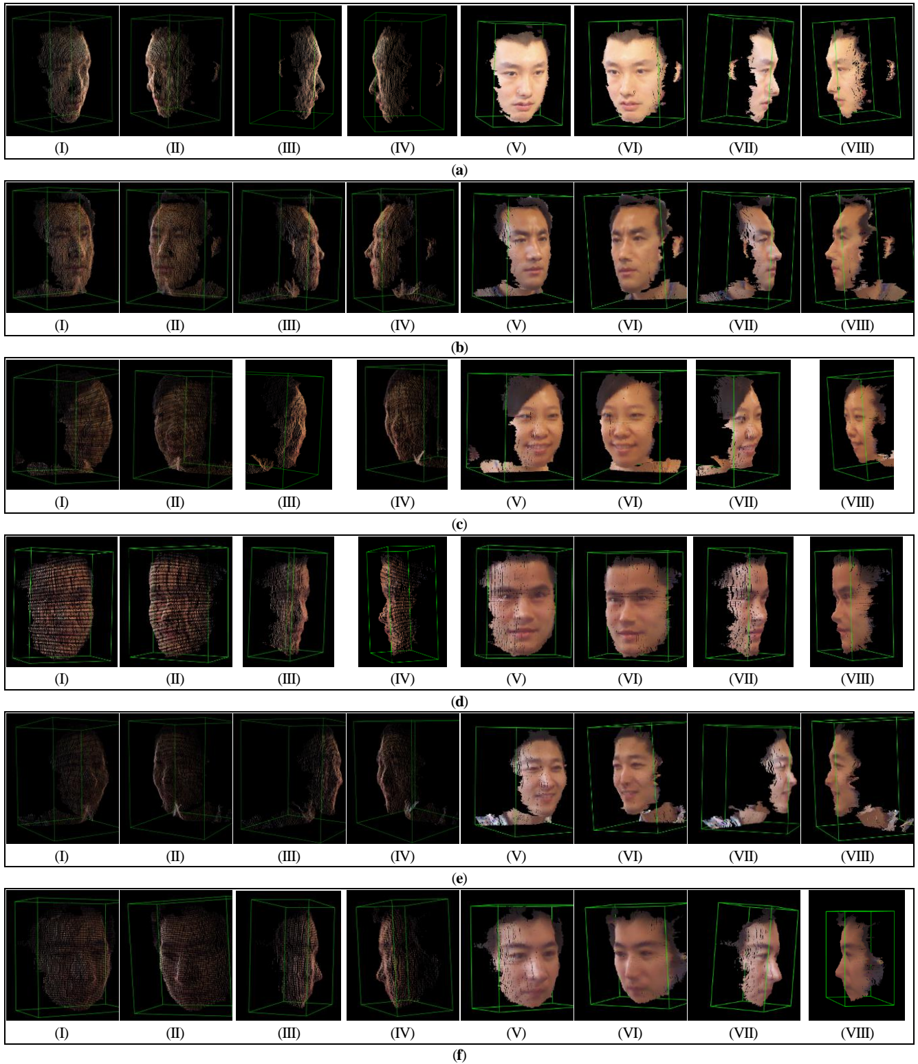
Fig. 8. Dense 3D facial point cloud producing results. (a) to (f) are six group of experiments with one subject in each group. In each group, (I) to (IV) are the initial 3D facial point cloud obtained after the first stage of proposed method, while (V) to (VIII) are the dense 3D facial point cloud obtained after final stage of the proposed method.
