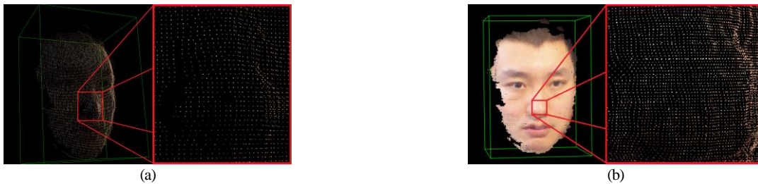
Fig. 7. Demonstration of the interpolation performance in the nose area. (a) The initial 3D facial point cloud achieved by the first stage; (b) The final dense 3D facial model obtained by the second stage. The nose area both in (a) and (b) is magnified for comparison.
