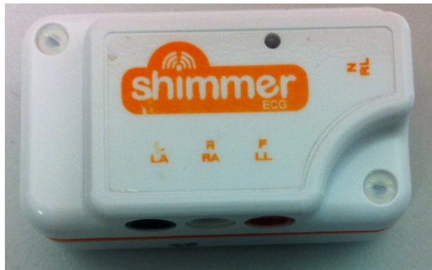
Figure 4.10: The mote with four connection ports with their connection label to each limb cable
