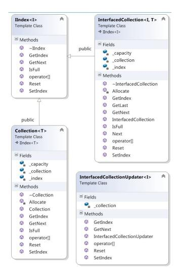
Figure 3.4: Class diagram showing the Memory Management classes
