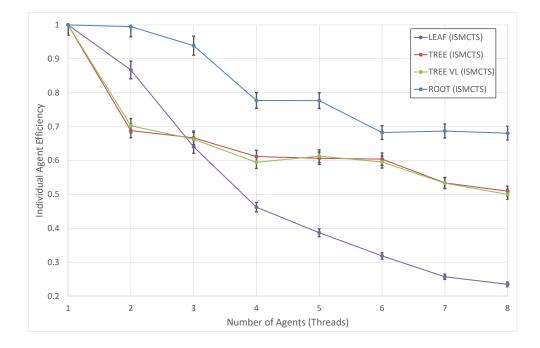
Figure 4.6: Results of applying four different parallelization techniques to ISMCTS operating upon state  $S_1$ . Results are expressed in individual agent efficiency.
