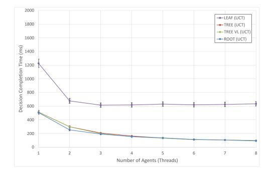
Figure 4.3: Results of applying four different parallelization techniques to UCT operating upon state  $S_1$ . Results are expressed in milliseconds used to complete a decision.
