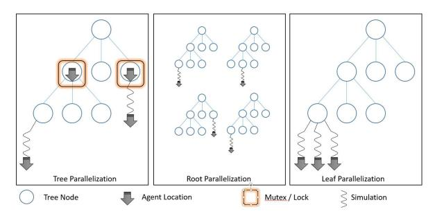
Figure 2.7: Overview diagrams for the most popular three parallelization methods
