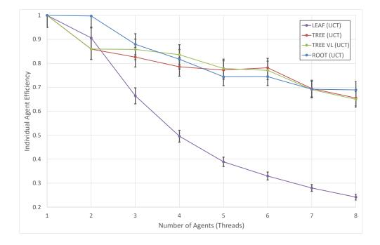
Figure 4.5: Results of applying four different parallelization techniques to UCT operating upon state  $S_1$ . Results are expressed in individual agent efficiency, where 1.0 represents optimal efficiency.
