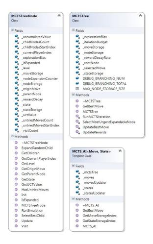
Figure 3.2: Class diagram showing the MCTS Tree class and associated sub-classes
