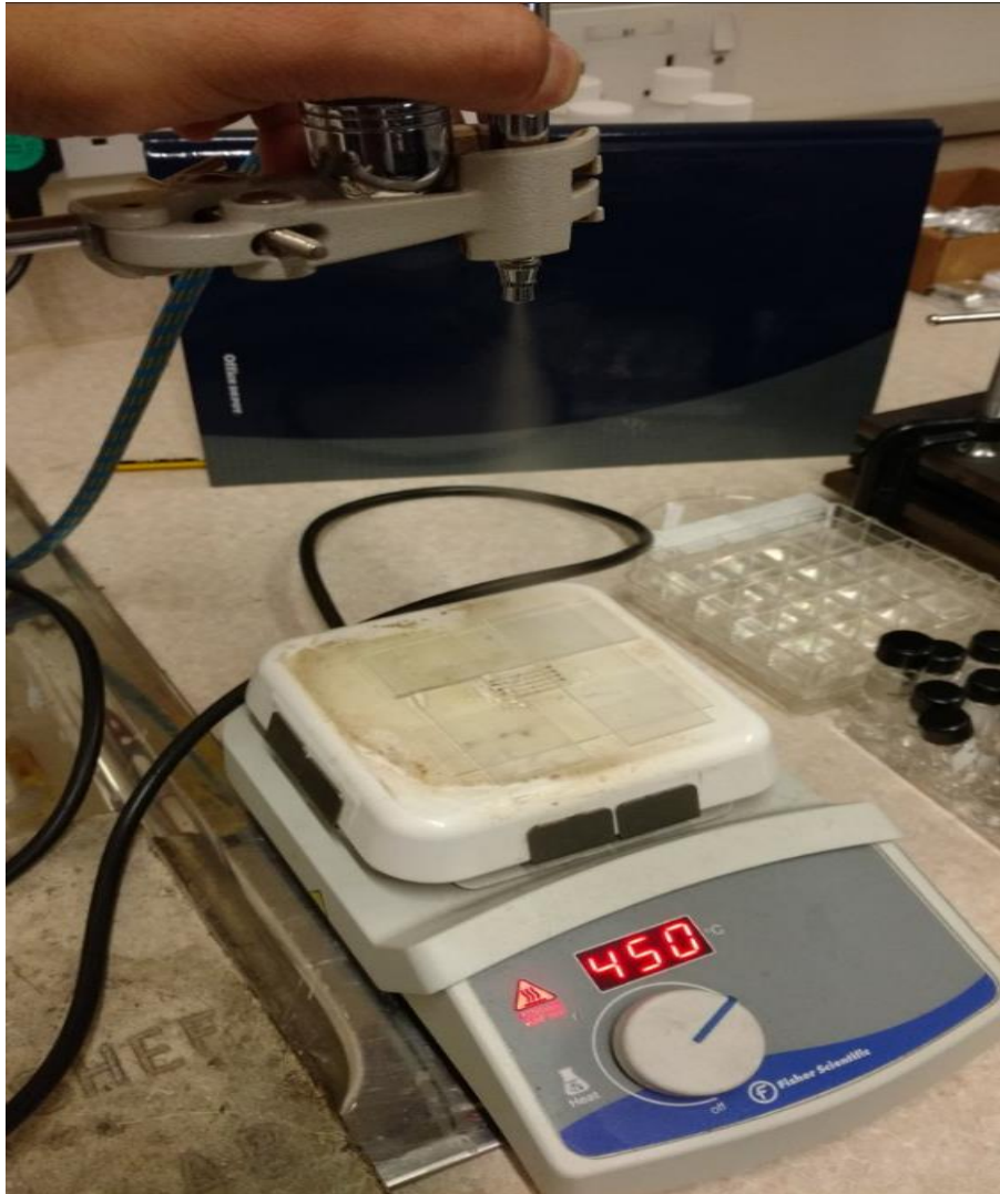
Figure 5-12: Picture of sprayed aqueous \text{ZnCl}_2 solutions onto heated (450 °C) TFT contact substrates.
