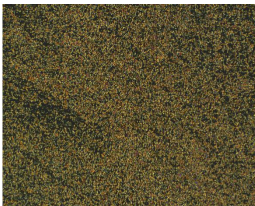
Figure 6.13: Photomicrograph of the smectic B phase of the 1:2 mixture of Compound 22 and its chloride salt at 128 °C.
