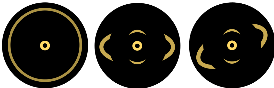
Figure 1.10: A cartoon representation showing the sharp small angle diffractions, as well as the diffuse wide angle diffractions. The rotation difference between the 'brackets' at wide angles in (b) and (c) show the tilt angle of the smectic C phase (c).
