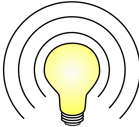
Figure 4: A spherical wavefront. Sources such as light-bulbs and stars, that emit waves in all directions, generate spherical wavefronts.
