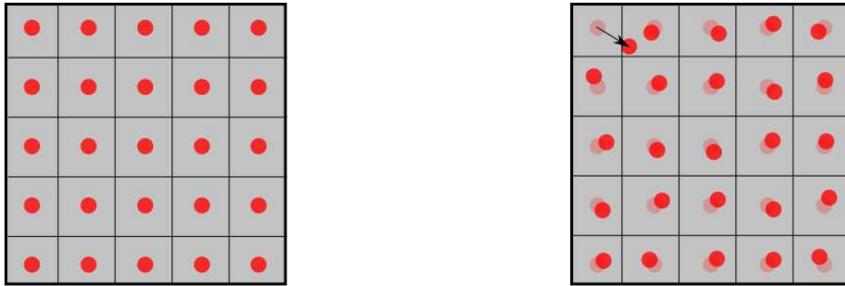
(a) Each spot is within the lenslet grid. (b) Large aberrations can cause gridding errors.
