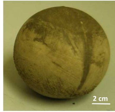
Fig. 2. Cement sphere after manufacture.
