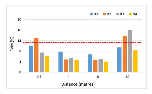
Figure 4.24 EVM of downlink **1x2 MRC-SIMO** measured at inter-RAU distance of 0.3m, 4m, 6m and 10m at different positions A1-A4 (top) and B1-B4 (bottom).
