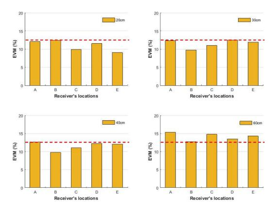
Figure 5.22 EVM result of 60GHz experiment at 20cm, 30cm, 40cm and 60cm transmit antenna separation distances using zero-forcing spatial multiplexing algorithm.
