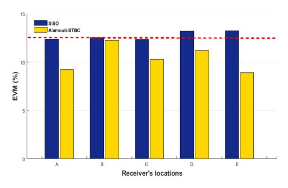
Figure 5.21 EVM result of SISO compared with the emulated 2x2 MIMO for 20cm transmit antenna separation at different receiver's locations using Alamouti STBC spatial diversity algorithm.
