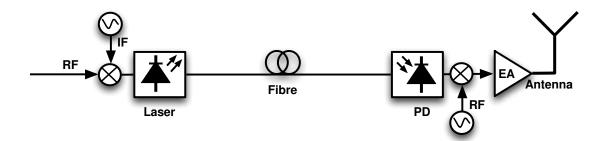
Figure 2.4 IF-over-fibre link.
