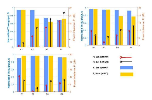
Figure 3.14 Throughput S and power imbalance Pi results of MIMO using set 2 and set 4
