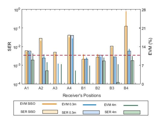
Figure 4.11 SER and EVM of downlink **2x1 TAS-MISO** measured at inter-RAU distance of 0.3m and 4m at different positions compared to **SISO**.
