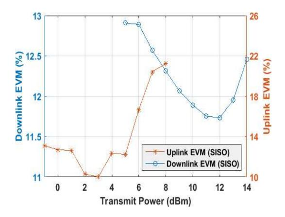
Figure 4.5 EVM of downlink and uplink signal transmitted from the RAU as the transmit power is increased to determine the optimum transmit power for measurement.
