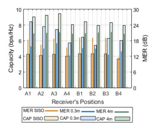
Figure 4.21 Capacity and MER of downlink **2x2 ZF-MIMO** measured at inter-RAU distance of 0.3m and 4m at different positions compared to **SISO**.
