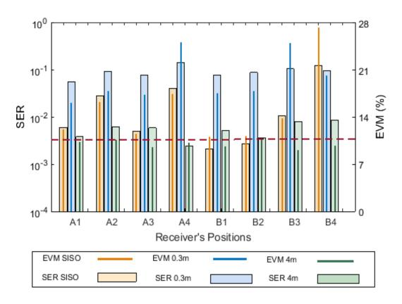
Figure 4.14 SER and EVM of downlink **2x2 ZF-MIMO** measured at inter-RAU distance of 0.3m and 4m at different positions compared to **SISO**.
