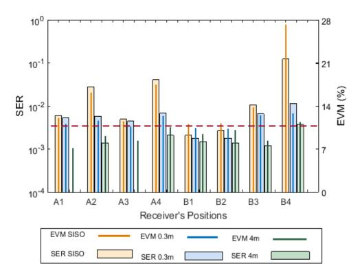
Figure 4.17 SER and EVM of downlink **2x2 DD/MRC-MIMO** measured at inter-RAU distance of 0.3m and 4m at different positions compared to **SISO**.
