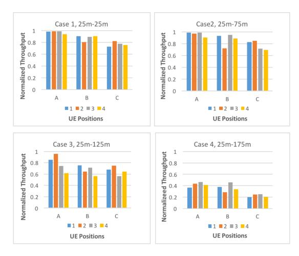
Figure 3.8 MIMO-supported downlink throughput with different fibre links (a) Case 1, 25m-25m (b) Case 2,25m-75m (c) Case 3,25m-125m (d) Case 4, 25m-175m.
