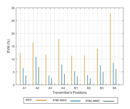
Figure 4.16 EVM of **SISO**, **Alamouti STBC-MISO** and **Alamouti STBC-MIMO** scheme measured at inter-RAU distance 4m at different positions A, B (1-4).
