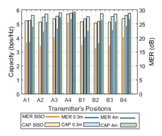
Figure 4.20 Capacity and MER of downlink **1x2 MRC-SIMO** measured at inter-RAU distance of 0.3m and 4m at different positions compared to **SISO**.
