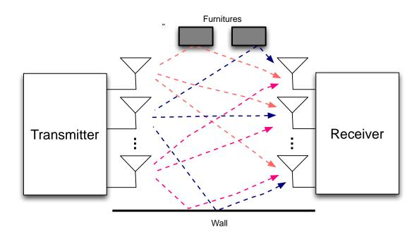
Figure 2.9 MIMO with multipath fading.
