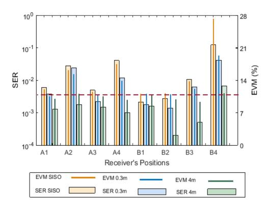
Figure 4.12 SER and EVM of downlink **2x1 DD-MISO** measured at inter-RAU distance of 0.3m and 4m at different positions compared to **SISO**
