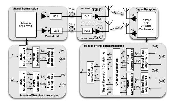
Figure 4.2 The downlink Experimental setup for 2x2 MIMO over Fiber EA= Electric amplifiers PD=Photodetector, LD=Laser diode, RAU=Remote antenna unit
