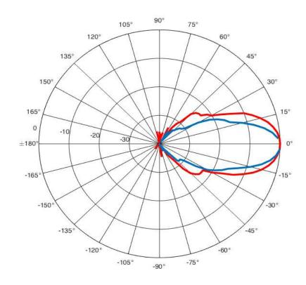
Figure 5.12 Radiation pattern of the two transmitting horn antennas.
