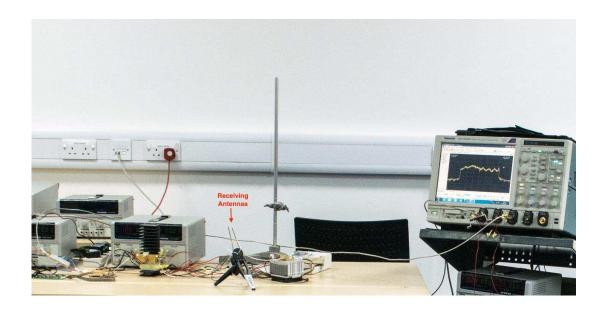
Figure 5.9 Receiving antenna connected to the differential baluns that produces I,  $\bar{I}$ , signal for the gRSC0016 60GHz receiver circuit and the signal captured at the Oscilloscope for offline processing.
