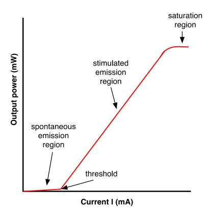
Figure 2.7 Laser P-I curve.
