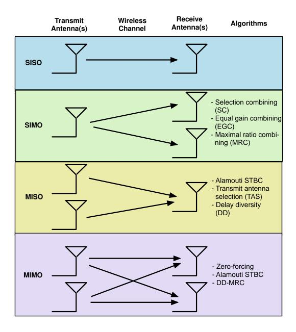
Figure 4.1 Description of SISO system and Multi-antenna configurations
