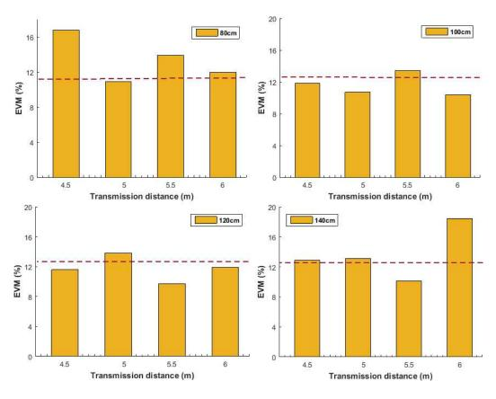
Figure 5.18 EVM result of 2x2 spatial multiplexing-MIMO for 80cm, 100cm, 120cm and 140cm transmit antenna separation distances at 4.5m, 5m, 5.5m and 6m wireless transmission distance.
