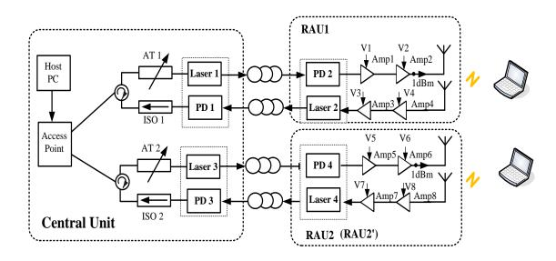
Figure 3.2 The experiment set-up. PD=Photodetector, AT=Attenuator, V=Voltage, ISO=Isolator, Amp=Amplifier.
