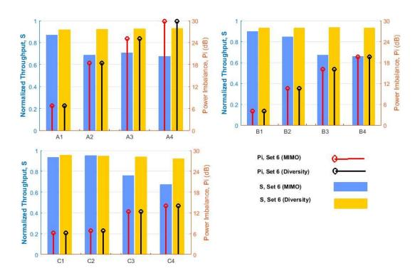
Figure 3.15 Throughput S and power imbalance Pi results of MIMO using set 6 and spatial diversity using set 6.
