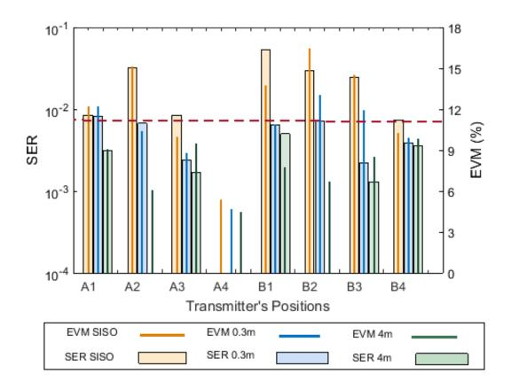
Figure 4.6 SER and EVM of uplink **1x2 SC-SIMO** measured at inter-RAU distance of 0.3m and 4m at different positions compared to **SISO**
