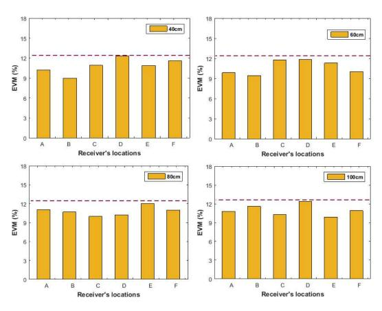
Figure 5.13 EVM result of 2x2 spatial diversity-MIMO at receiver location A to F for 40cm, 60cm, 80cm and 100cm transmit antenna separation distances at 3m wireless transmission distance.
