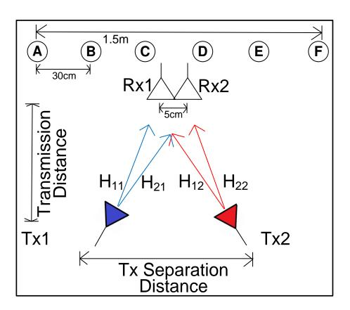
Figure 5.3 Measurement layout of the testing room.
