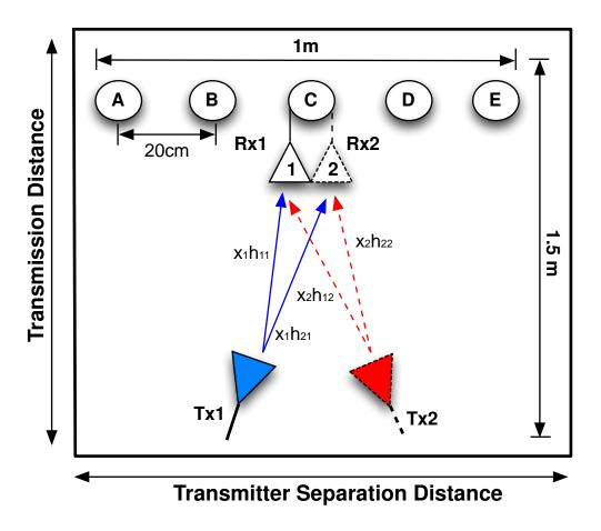
Figure 5.11 Measurement layout of 60GHz experiment
