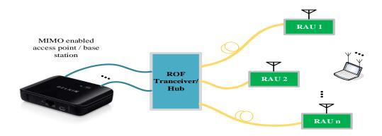
Figure 2.14 Diagram showing 2x2 MIMO over RoF DAS.
