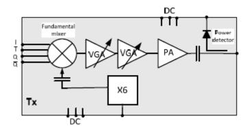
Figure 5.7 gTSC0020 60GHz integrated transmitter circuit [12].
