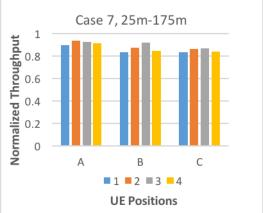
Figure 3.10 Spatial Diversity-supported downlink throughput with different fibre link lengths (a) Case 6, 25m-25m (b) Case 7, 25m-175m
