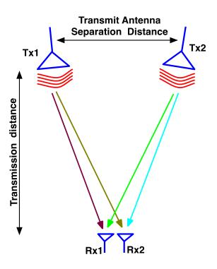
Figure 5.1 MIMO in Line-of-sight (LOS) propagation.
