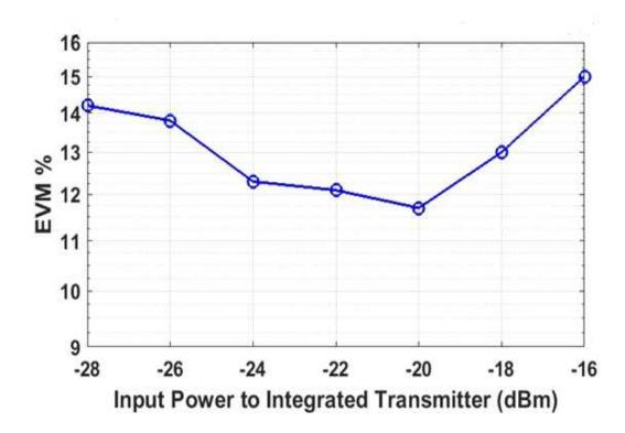
Figure 5.10 EVM result showing the performance of the 60 GHz integrated transmitter at different IF power levels.
