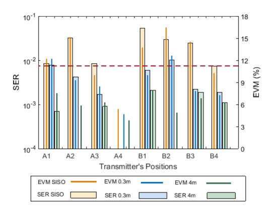
Figure 4.7 SER and EVM of uplink **1x2 EGC-SIMO** measured at inter-RAU distance of 0.3m and 4m at different positions compared to **SISO**.
