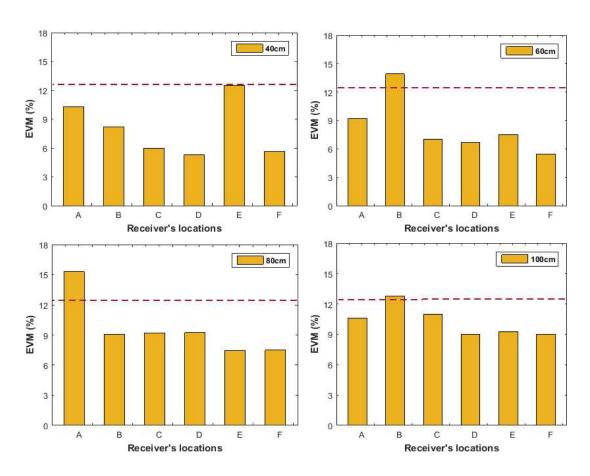
Figure 5.14 EVM result of 2x2 spatial diversity-MIMO at receiver location A to F for 40cm, 60cm, 80cm and 100cm transmit antenna separation distances at 3.5m wireless transmission distance.
