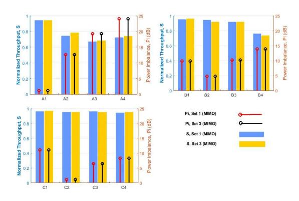
Figure 3.13 Throughput S and power imbalance Pi results of MIMO using set 1 and set 3
