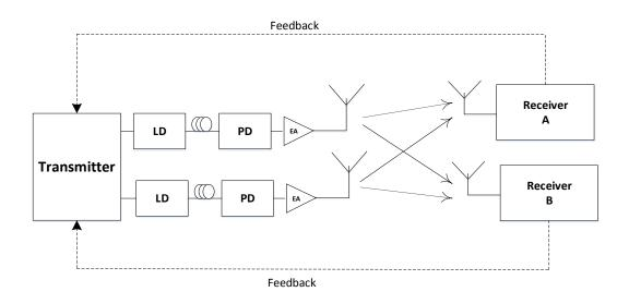
Figure 6.1 An example of the experimental setup of a multi-user pre-coding MIMO in RoF-DAS.
