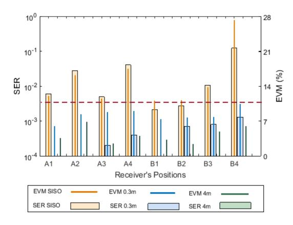
Figure 4.15 SER and EVM of downlink **2x2 Alamouti STBC-MIMO** measured at inter-RAU distance of 0.3m and 4m at different positions compared to **SISO**.
