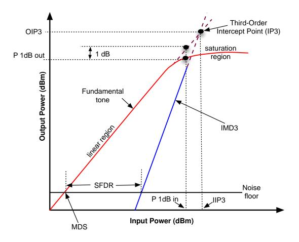
Figure 2.8 Typical plot of output power against input power for an analogue RF system, showing third-order intercept point, spurious-free dynamic range and 1-dB compression point.
