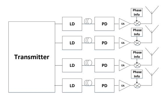
Figure 6.2 An example of the experimental setup of an analogue beamforming in RoF system.
