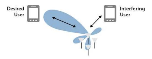
Figure 2.12 Smart antenna system - beamforming [22].
