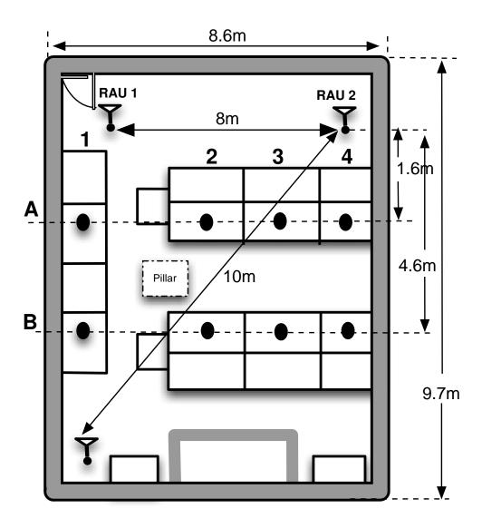
Figure 4.3 Testing room layout, an open plan office. A, B (1-4) represent the positions of the mobile user (the Oscilloscope/AWG)
