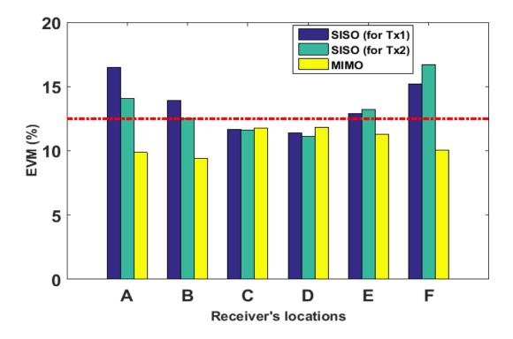
Figure 5.16 EVM results of  $2\times2$  spatial diversity-MIMO using Alamouti STBC at different user locations compared with the performance of SISO system.
