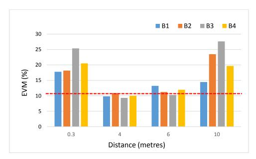
Figure 4.25 EVM of downlink **2x2 ZF-MIMO** measured at inter-RAU distance of 0.3m, 4-m, 6-m and 10-m at different positions A1-A4 (top) and B1-B4 (bottom).
