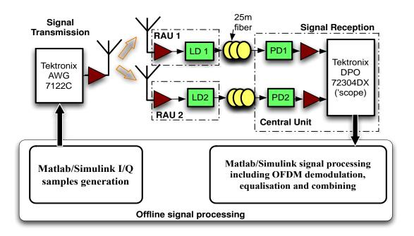
Figure 4.4 The uplink experimental setup for 1x2 SIMO over Fibre
