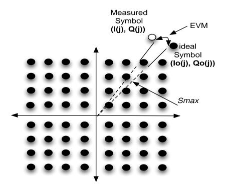
Figure 2.13 Constellation diagram of 64-QAM.
