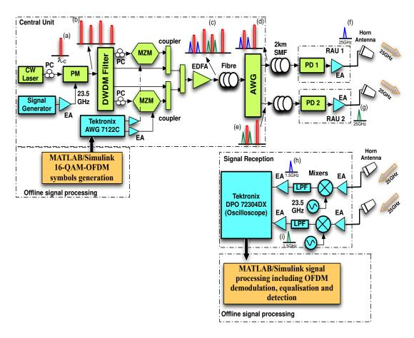
Figure 5.2 Experimental set-up for 25GHz RoF-transported 2x2 MIMO system CW Laser – Continuous-wave Laser, PM- phase modulator, DWDM filter – dense wavelength division multiplexing filter, EA= Electric amplifiers, MZM –Mach-Zehnder modulator, EDFA- Erbium Doped Fiibre Amplifier, AWG - Array Waveform Grating, PD=Photo-detector, RAU=Remote antenna unit, LPF – low pass filter
