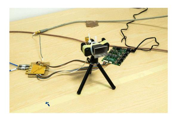
Figure 5.6 IF signal fed into a differential baluns that produces I,  $\bar{\mathbf{I}}$ , for the gTSC0020 60GHz integrated transmitter circuit and wirelessly transmitted through an horn antenna.
