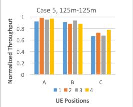
Figure 3.9 MIMO-supported downlink throughput with the equal fibre link lengths (a) Case 1, 25m-25m (b) Case 5, 125m-125m
