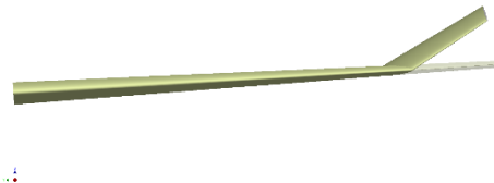
Figure 4. Front view showing positive fold angle for a hinge angle of 30^\circ .
