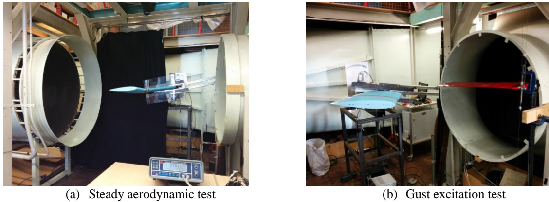
Figure 8. Wind tunnel test set-up
