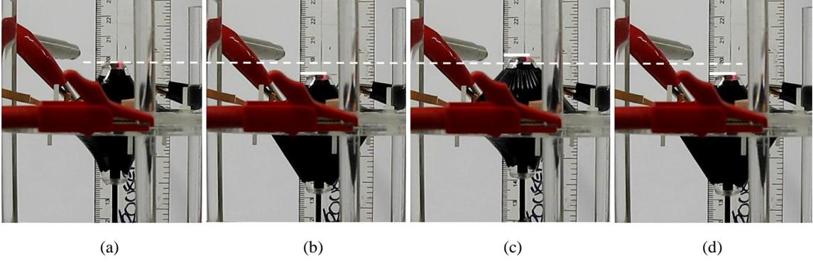
Figure 6. Motion of the spacer (and load) when top and bottom cone DEAs are alternatively actuated. (a) to (d) shows the movement of the central spacer (also the load) under an alternating square driving voltages with an amplitude of 3 kV. Under 45 g load ( $\sim 5$  times the weight of actuator), the actuator is able to provide a stroke of 10.4 mm (4.8 mm upwards and 5.6 mm downwards), equaling to 23.6% of its height.
