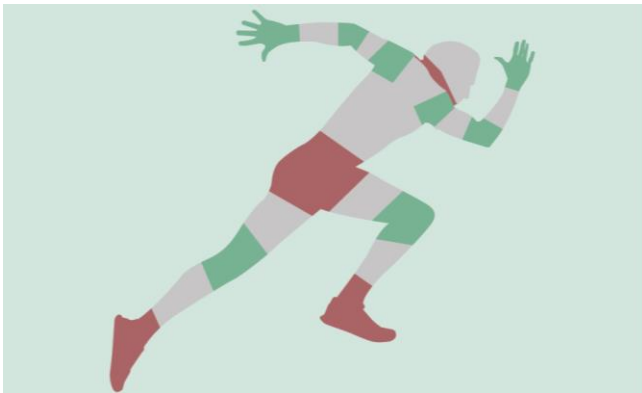
Figure 2. Ideal placements of the changeable stiffness patches: green are the best positions; gray unnecessary; red potentially dangerous.
