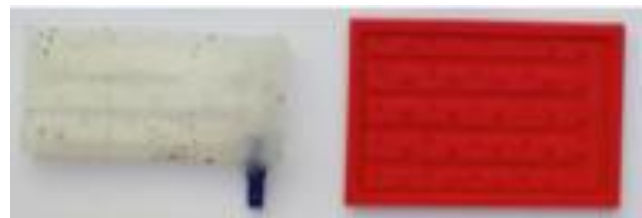
Figure 12. (Left) Patch with channels (filled with flour for better visual). (Right) 3D printer mold used to generate the bladder with silicon.
