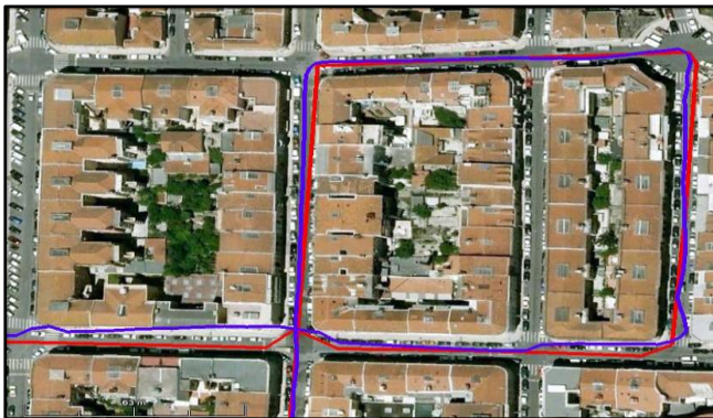
Figure 7: Google Earth view of the results with linear regression in linear crossroads. In blue the GPS estimates and in red the constrained Kalman filter solution.
