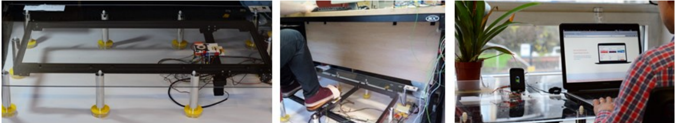
Figure 1. Left: CoilMove is an actuated surface to transfer energy to the body, allowing wearable and mobile computing devices to be charged whilst remaining on the body. Middle: CoilMove transferring energy to a user's foot in one of the characterization experiments. Right: CoilMove locates devices based on the presence of a magnet and could additionally support devices resting on the surface, as well as devices on the body.
