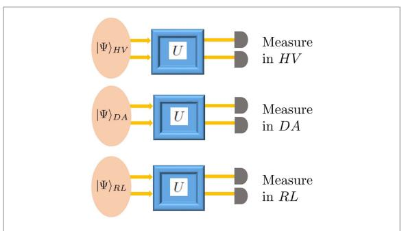
Figure 2. Single run of the multi-parameter estimation protocol investigated in [11]. Begin with three input states  $|\Psi\rangle_{HV}$ ,  $|\Psi\rangle_{DA}$ ,  $|\Psi\rangle_{RL}$ . These are passed through the unitary U before being respectively measured in bases HV, DA and RL.
