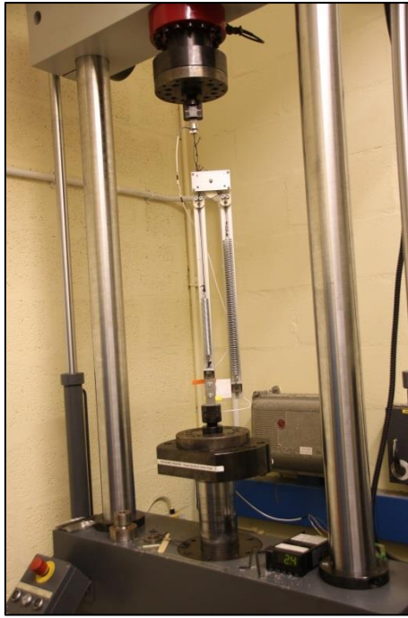
Figure 15. SPNS mechanism installed on material test machine
