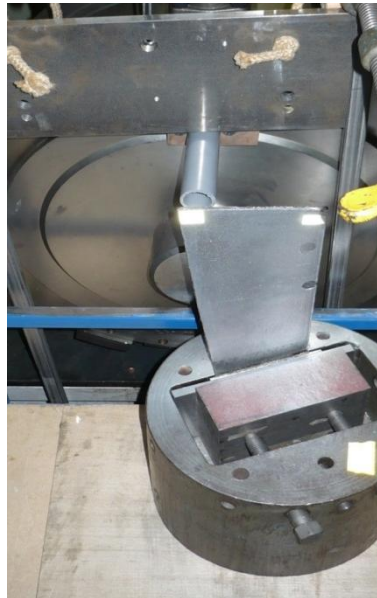
Figure 5 Text fixture, blade and exciter's nozzle
