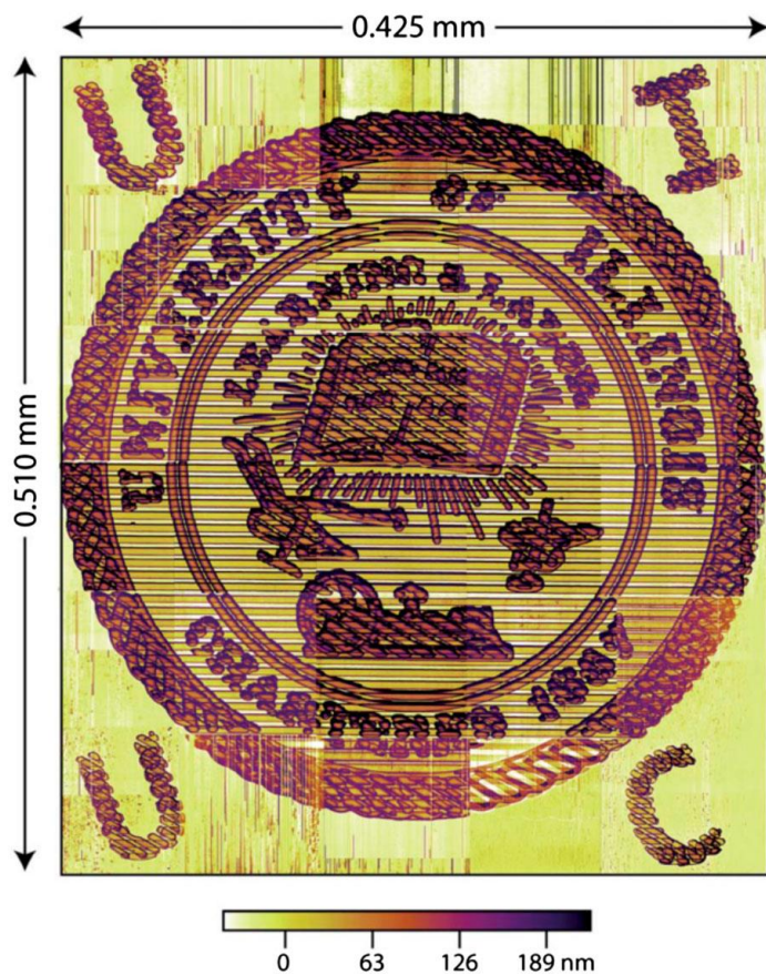
Figure 9 Composite HS-AFM image collected by Seong et al. 145 using a custom cantilever chip consisting of 30 heat sensitive cantilevers in parallel
