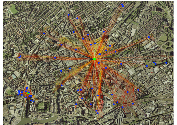
Fig. 3. Modelling of MPCs for 3-D MU-MIMO in a sectorised Macrocell and Picocell (green dots: BS locations, blue dots: UE locations)
