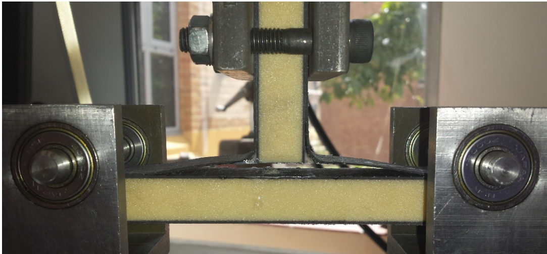
4 Fig. 4. T-joint tensile test set up. Delamination along overlamine/substrate interface of repaired 5 vascularised T-joint sample (T2) 6 7 8 9 10 11 12
