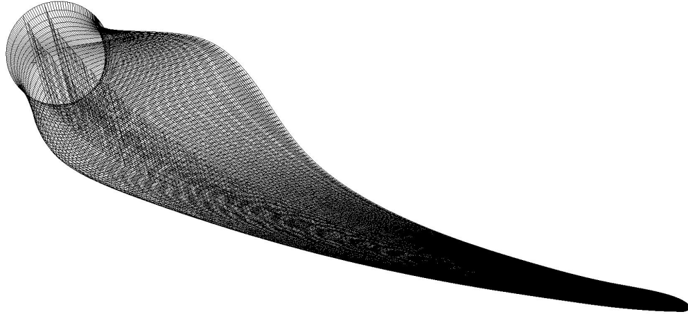
Figure 10: Finite Element model, full blade structure
