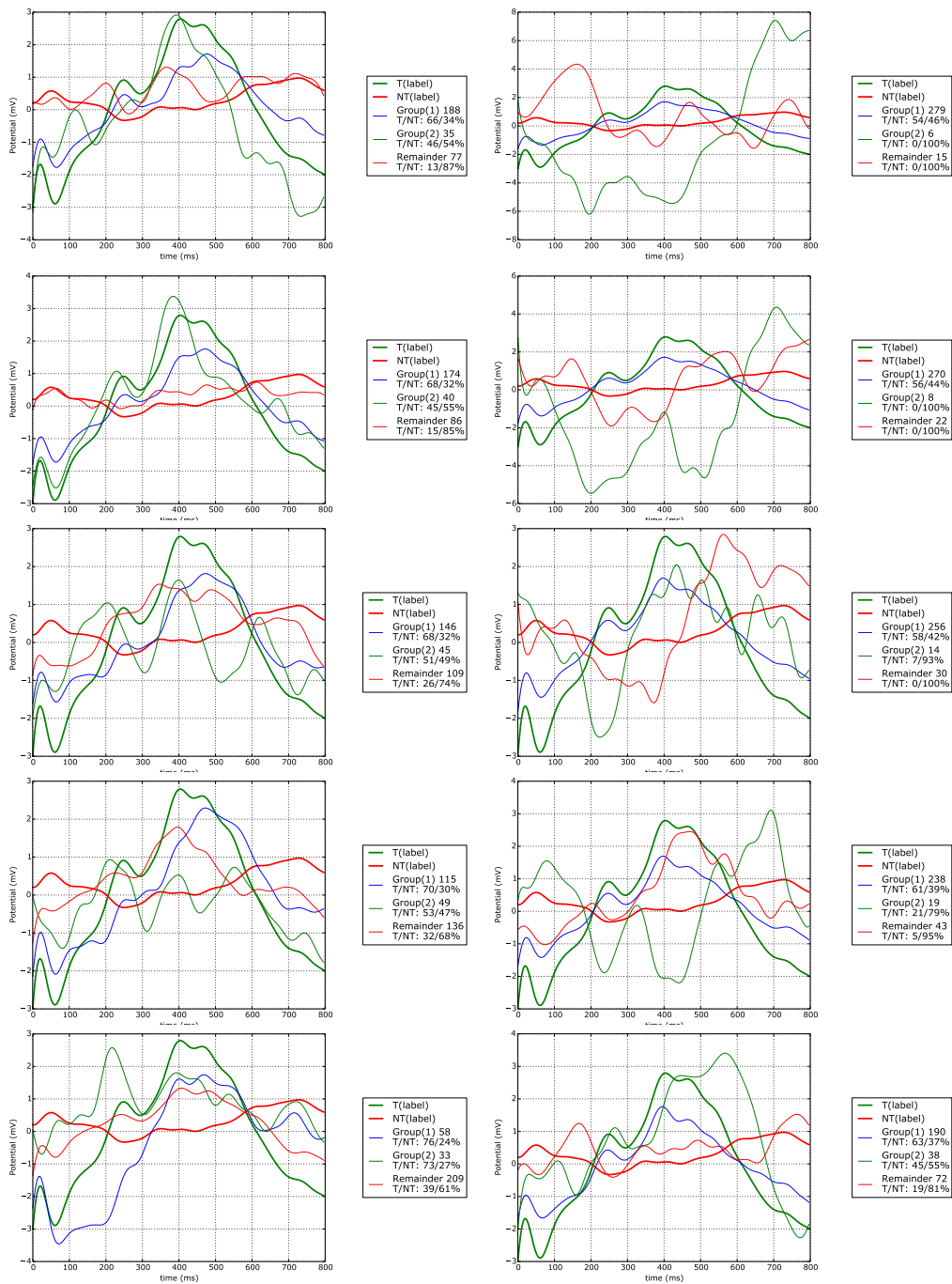
Figure B.25: Extracting two groups of epochs using the Kruskal-Wallis test. On the left V, right dV. Showing results for participant 9
