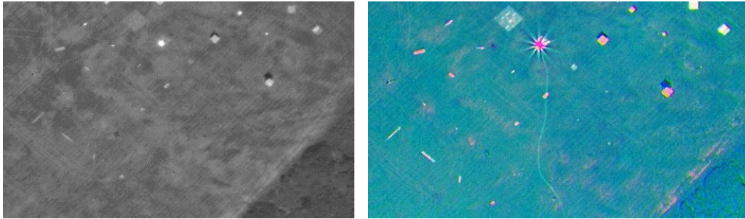
Figure 7: A pair of images showing the debris field. The intense specular reflection has generated a trailed image artefact in the CCD readout software used to create it.
