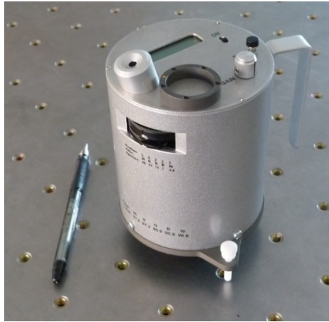
Figure 17. Picture of the multiple wavelength reflectometer 15R-RGB by D&S.
