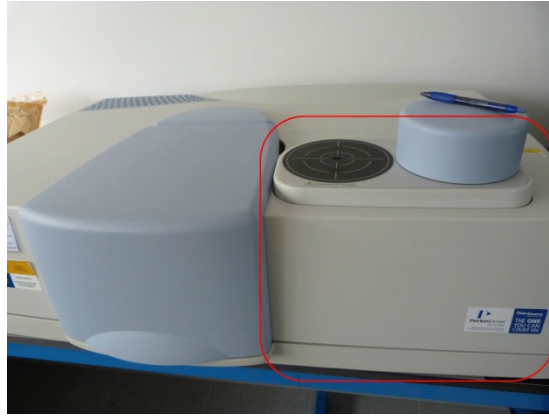
Figure 5. Picture of the spectrophotometer Lambda 1050 by PE with the URA. The red square indicates the URA accessory, which is interchanged with the detector compartment (see Figure 2).
