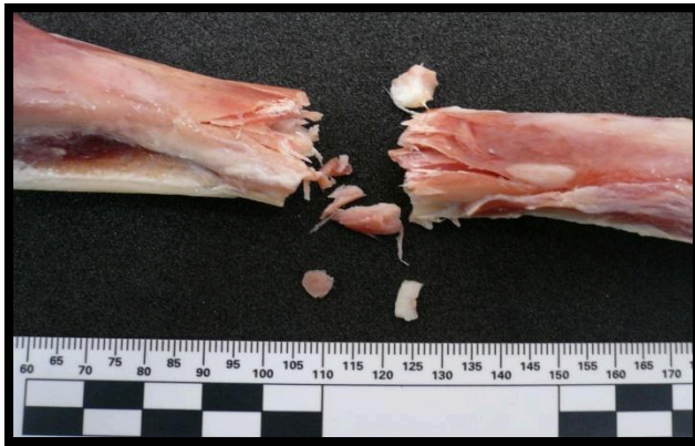
Figure 12 – Example of complete fracture in BFT 1
