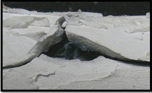
Figure 21 – Example of splintering effect in BFT 7
