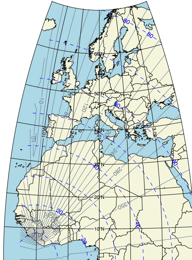
Figure 4 Contours of maximum azimuth speed ( \text{m s}^{-1} ) and local incidence angle for a GEO SAR satellite with a circular orbit, inclination 7.5^\circ , positioned at longitude -10^\circ .
