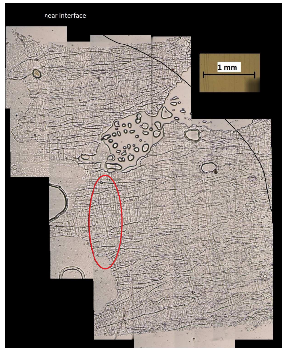
Figure 7: Microstructure of the longitudinal cut of ice built on a mirror polished surface finish titanium alloy substrate ( T=-15^{\circ}\text{C} , \text{LWC}=0.3\text{ g.m}^{-3} , V=80\text{ m.s}^{-1} , \text{MVD}=20\text{ }\mu\text{m} )
