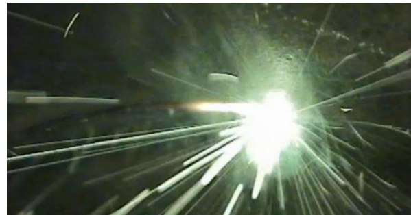
Figure 16: Root formation at 8.2 kW of laser power and 11.8 kW arc power (WFS 20 m/min)
