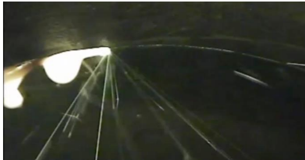
Figure 6: Root formation at 7.7 kW of laser power and 7.4 kW arc power (WFS 12 m/min)
