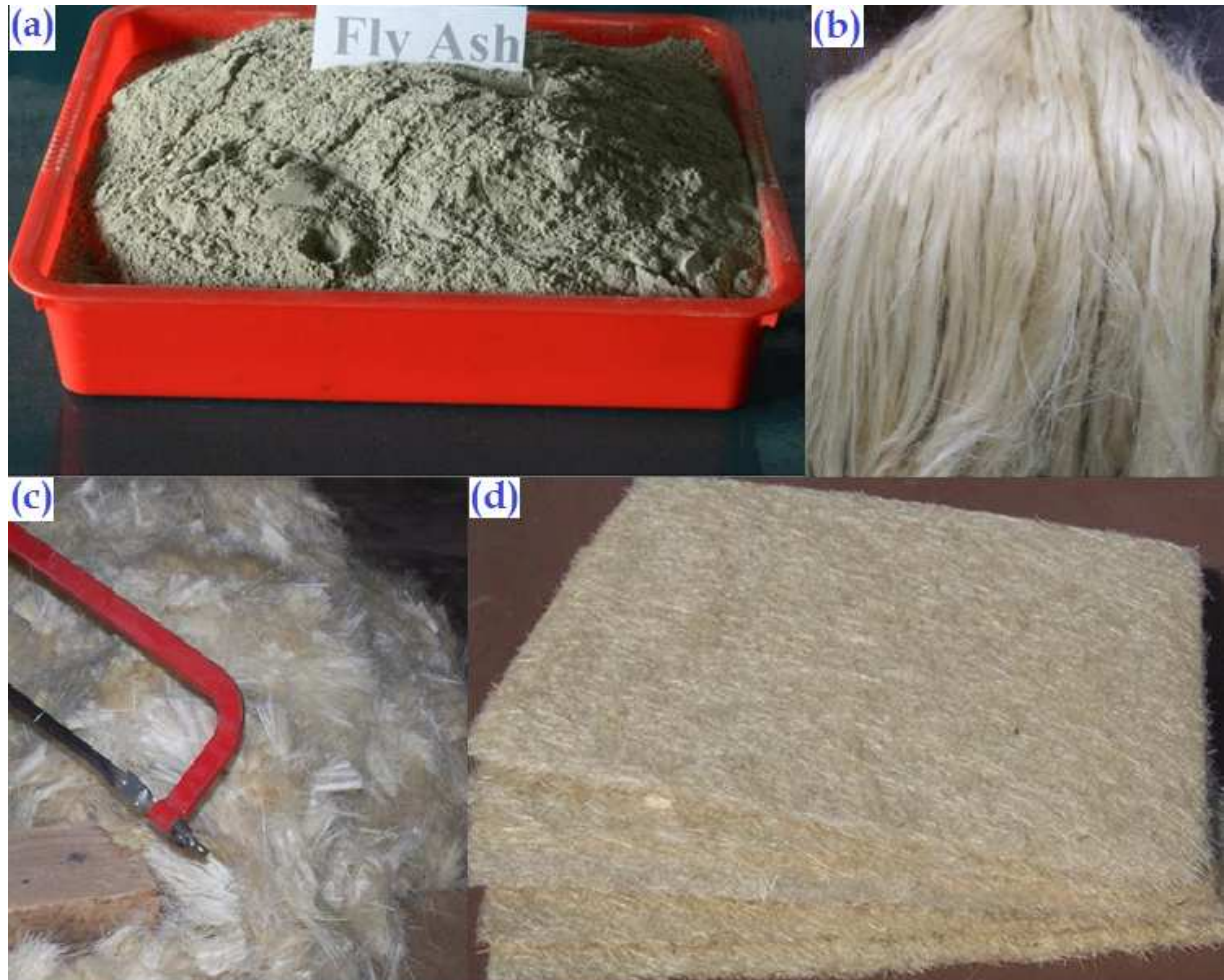
Fig. 1(a) Fly ash of STPC, Sarni, Madhya Pradesh, India (b) Processed sisal fibres from CSIR-AMPRI Bhopal, India (c) Processed sisal fibres cut into about 3.5 cm length 3-4 cm (d) Perform mats fabricated out of sisal fibres
