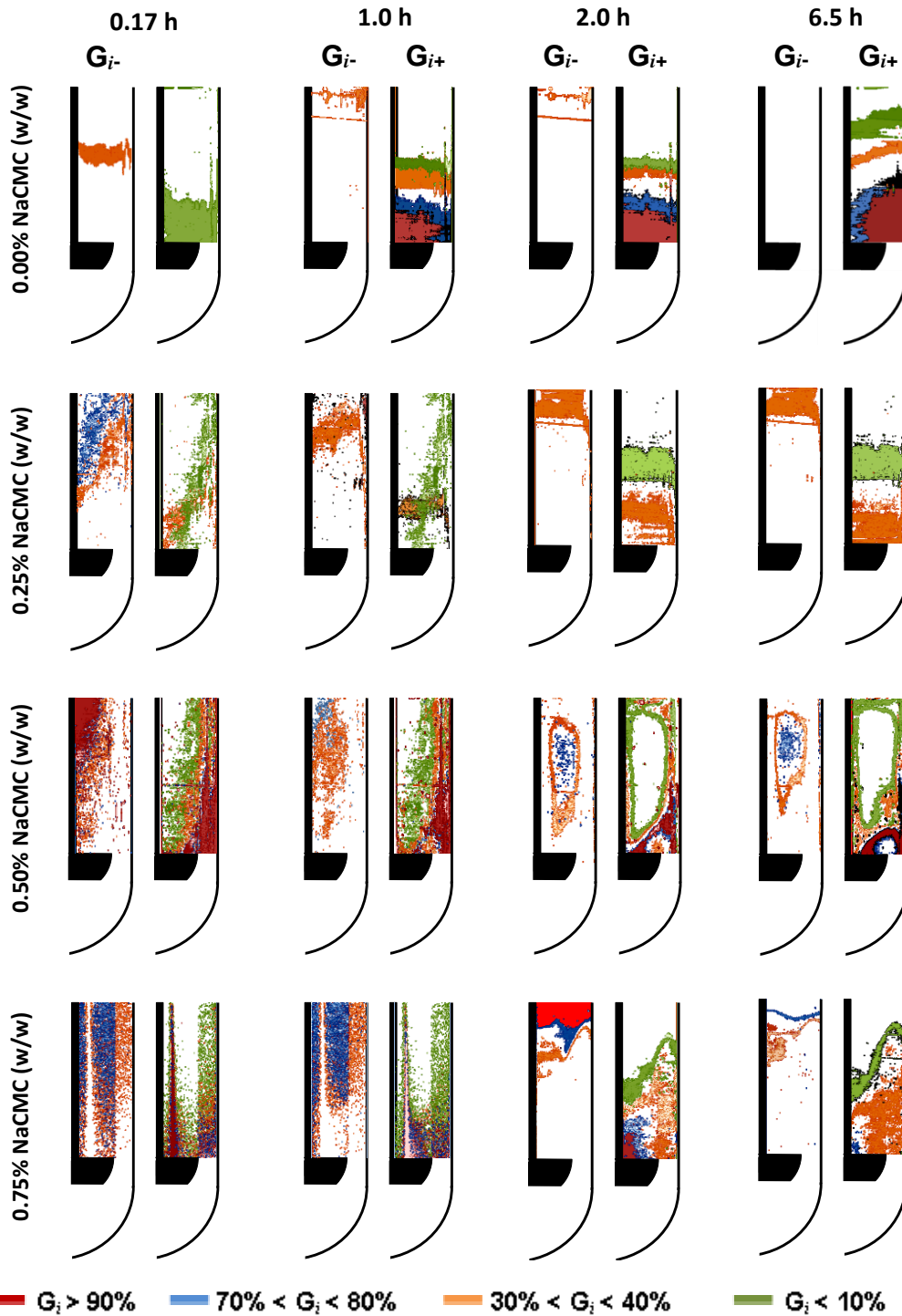
Figure 4.7. Illustration of striations detected using the individual striation method for selected ranges of level of mixedness, G_i , for (a) “simple buffer”; (b) 0.25% NaCMC (w/w); (c) 0.50% NaCMC (w/w); (d) 0.75% NaCMC (w/w).
