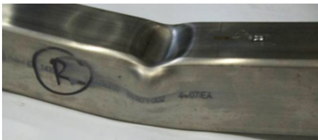
Figure 2.10: Local buckling failure mode (Theofanous and Gardner, 2010; Shi et al., 2014b).
