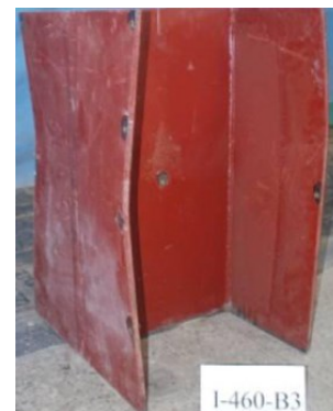
Figure 2.10: Local buckling failure mode (Theofanous and Gardner, 2010; Shi et al., 2014b).
