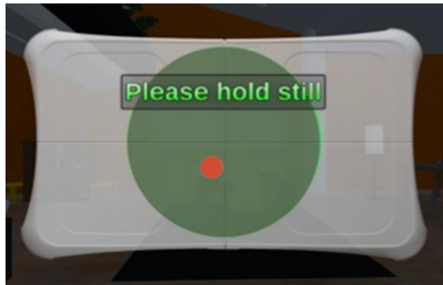
Figure 10: A screenshot taken of the calibration phase which was implemented prior to each block of new trials. This figure illustrates a red dot, which signifies an individual's COP. Individuals would shift their weight in response to the location of the red dot, aiming to get it at the cross hair in the middle. This procedure provided direct feedback to the individuals about their balance to ensure that at the start of trials, each individual was as close to their postural equilibrium as they could be.
