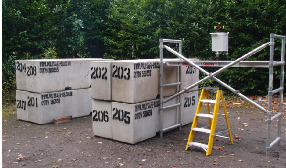
Figure 6.1: Photograph of the experimental set-up used. Showing the Scintrex CG-5 on top of the scaffold tower, with the Leica 360 degree prism on top, next to the two concrete anomalies.
