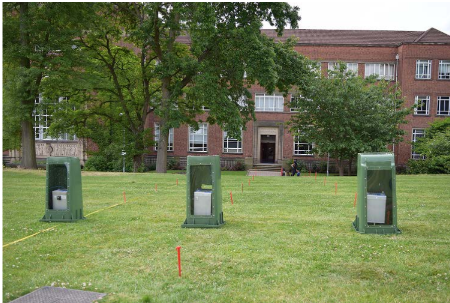
Figure A.2: Three Scintrex CG-5 instruments protected from wind noise by shielding.
