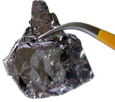
Figure 3.1: A large sample of \text{MoS}_2 with an approximate size of 15 \times 20 \text{ mm} [36].
