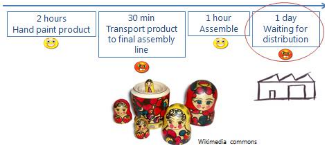
Figure 15 Value Stream Mapping and Just In Time concepts with an example from the Matryoshka dolls factory
