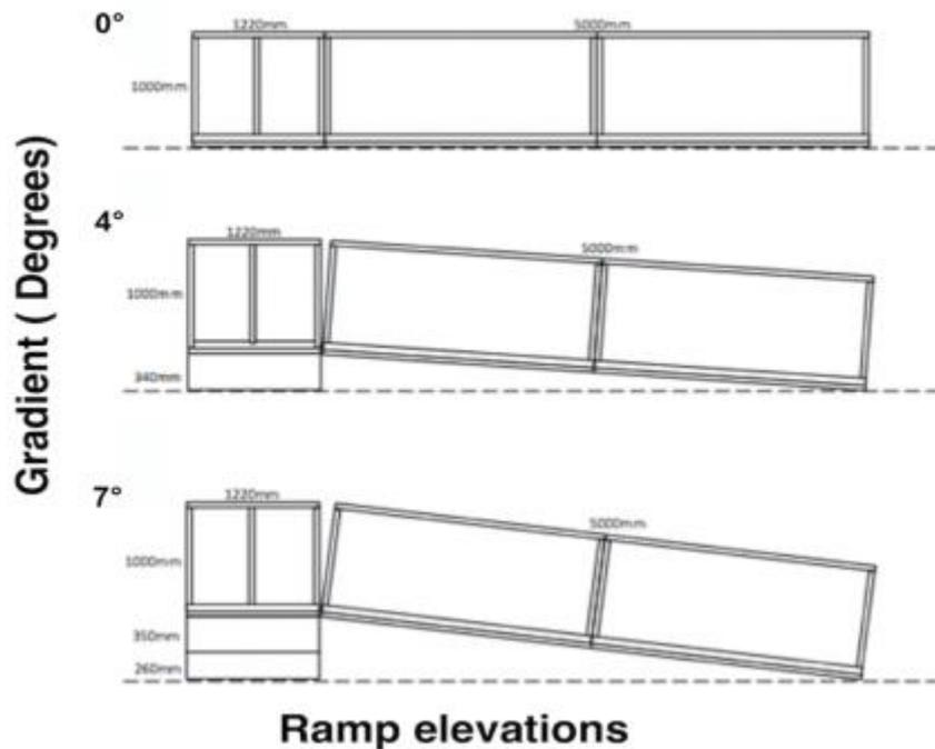
Figure 1. Custom-made wooden ramp elevations at 4 and 7 degrees.
