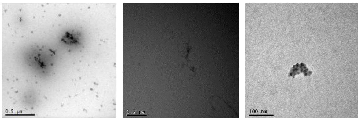
Figure 4.20 TEM images of 10 K PVP capped copper oxide nanoparticles.
