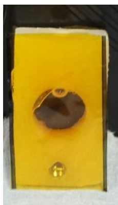
Figure 3.18 Teflon cell sealed with Kapton tape loaded with PVP capped metal oxide nanomaterial dispersion.
