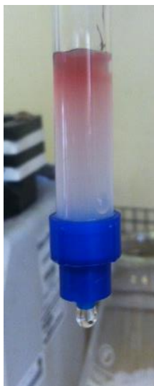
Figure 3.10 Sephadex size exclusion column showing the non-thiolated DNA coated particles are unable to pass through the column
