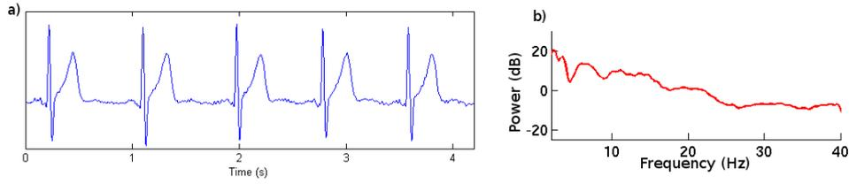
Figure 4.7: A sample of ECG artefact component; a repeating pattern of peaks generated by heart beats over time (a) and higher power spectrum at low frequencies (b).
