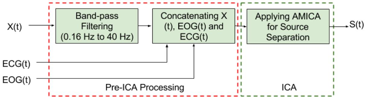
Figure 3.10: Block diagram of the obtained optimum pre-processing steps, where the raw EEG signal  $X(t)$  is band-pass filtered at  $0.16Hz - 40Hz$ , and concatenated with ECG and EOG channels. Then the AMICA algorithm is employed to separate the independent sources,  $S(t)$ .
