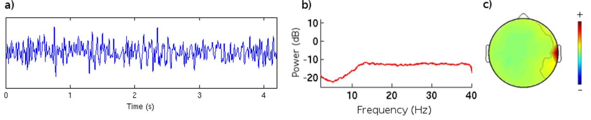
Figure 4.5: A sample of muscle artefact; high frequency activation of muscle IC over time a); higher spectral power above  $20Hz$  b); and the concentrated activity of the muscle artefact around a few electrodes on the scalp c).
