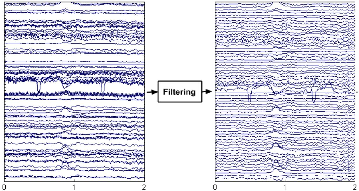
Figure 3.4: Not filtered EEG data (left) versus band-pass filtered EEG data with high cut-off frequency of  $40Hz$  (right).
