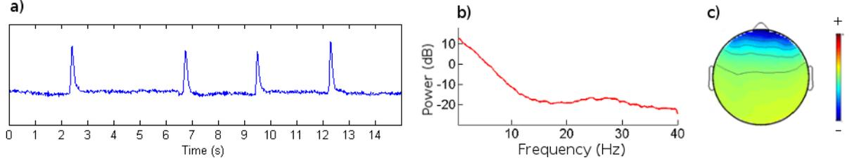
Figure 4.1: A sample of typical blink artefact; the high amplitude voltages generated by blinking over time (a); higher spectral power below  $5Hz$  (b); and the effect of blinking on electrodes positioned in frontal area on the scalp (c).
