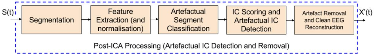
Figure 4.14: Block diagram of the proposed automatic artefact detection method. First, the ICs are segmented and the features (described in section 4.2.1) are extracted from each segment. Then, the segments are classified into artefact and non-artefact. Based on the result of this classification, artefact ICs are scored and detected. Finally, the detected artefact ICs are removed and the cleaned EEG,  $X'$ , is reconstructed.
