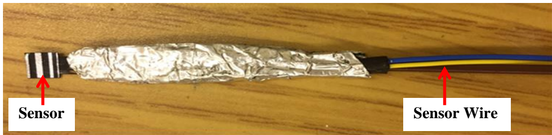
Figure 3.14: A photograph of 0.005 \times 0.005 \text{ m}^2 Radiant flux sensor [186].
