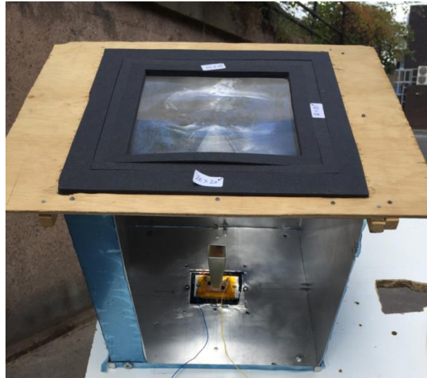
Figure 3.4: Controlling the GCR by controlling the Fresnel lens exposed area to the sun light.
