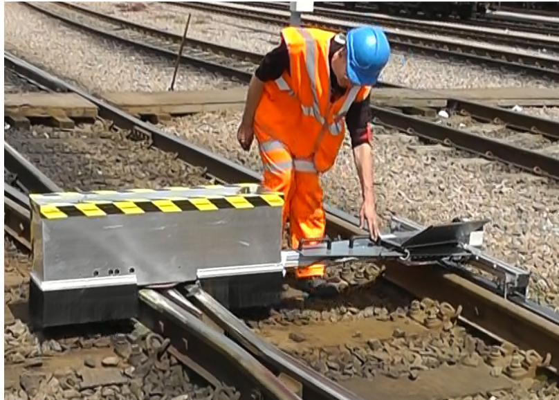
Figure 6-1 The developed S&C laser-based trolley on a measured railway crossing
