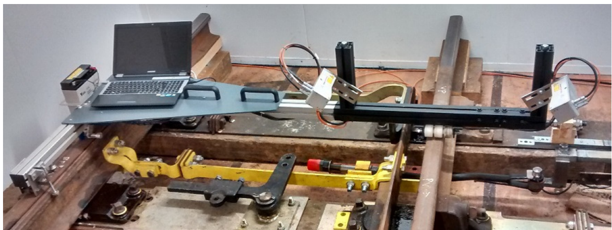
Figure 4-14 S&C inspection trolley
