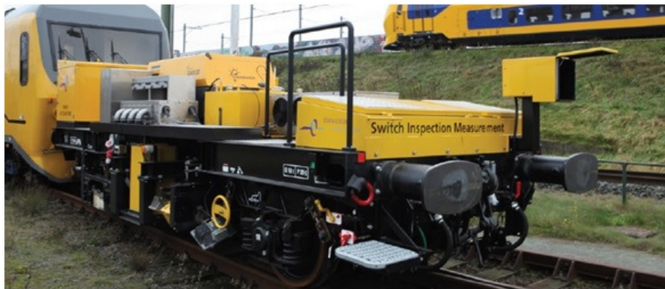
Figure 2-3 Switch Inspection & Measurement (SIM) wagon Courtesy and Copyright Eurailscout
