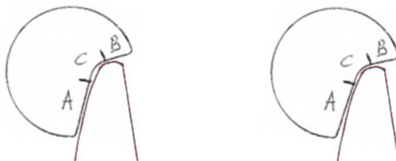
Figure 5-51 Example of how rocking of switch rail radius gauge may lead to different inspection results (left: pass example; right: fail example)
