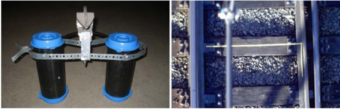
Figure 2-12 Overhead line mounted CCD camera prototype (left) and sample image (right) Courtesy and Copyright Matthias Asplund
