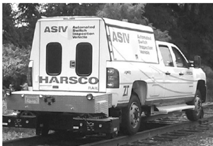
Figure 2-5 Automatic Switch Inspection Vehicle (ASIV) Courtesy and Copyright ZETA-TECH
