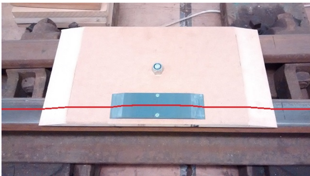
Figure 6-5 Reference board with known dimensions
