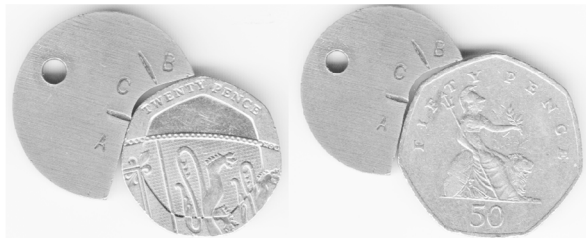
Figure 5-54 Switch rail radius gauge applied on a 20 pence and 50 pence coin
