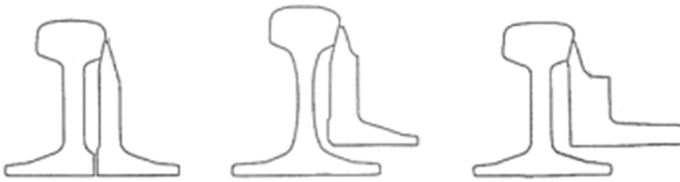
Figure 5-17 Switch planing used throughout NR railway infrastructure (left: 113 curved chamfered; centre: UIC60 shallow depth; right: 113A/UIC54B shallow depth)
