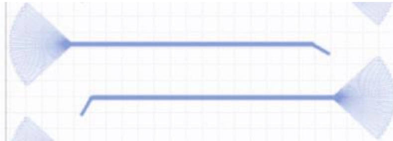
Figure 4.9 Layout of the FPCB interconnections to connect the electronic driving system with the ultrasound transducer array
