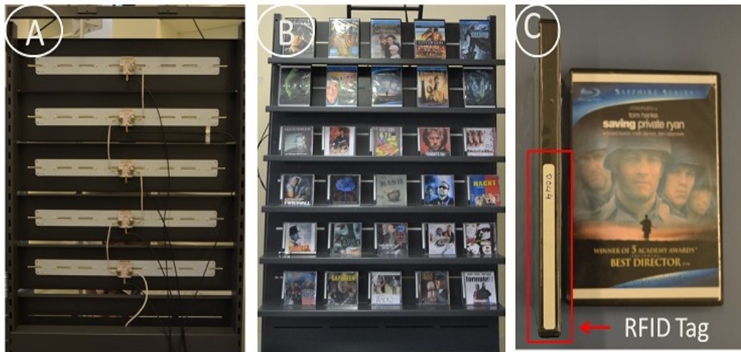
Figure 3. A) Back of a Smart Shelf showing the RFID System. B) Frontal view of shelf with RFID-tagged products. C) Product showing RFID Tag.
