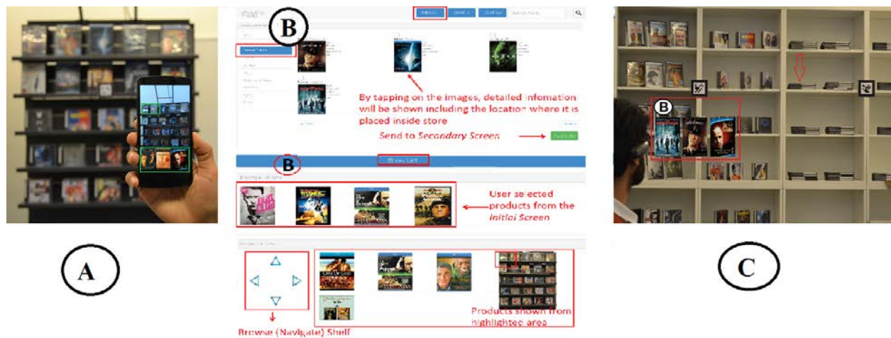
Figure 4. A) Handheld device AR Interface. B) Touchscreen Web Interface. C) Smart Glass AR Interface
