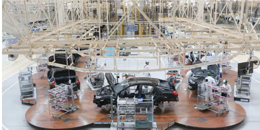
Fig. 1. U-line configuration at Honda's car assembly plant 1
