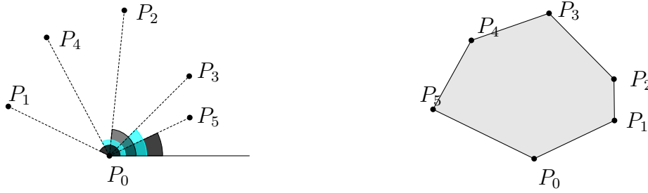
Figure 5.7: Convex polygon construction. The left image shows a set of points randomly organized and the angle with respect to the horizontal ray with origin P_0 . The right figure is the result of ordering the points by increasing angles.
