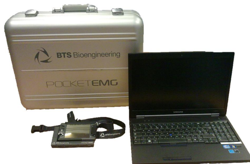
Figure 3.1 Pocket EMG medical device used to measure the electrical activity of the muscles near to the skin.
