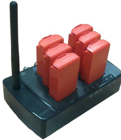
Figure 3.2 Six inertial measurement units docked in an Awinda station; they were used to measure the elbow kinematics.
