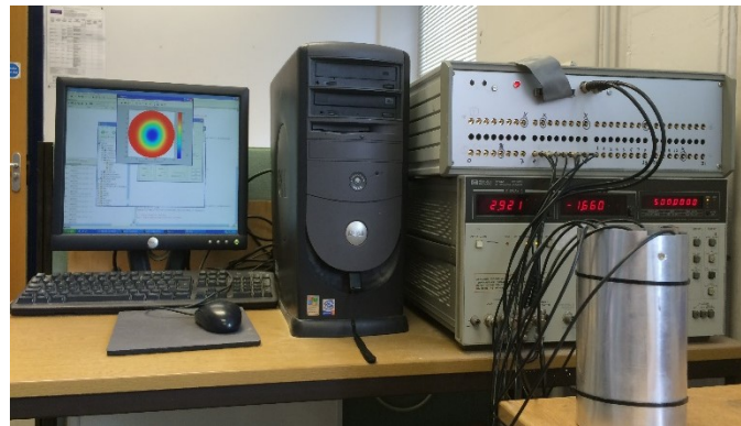
Figure 18 Impedance analyser based ECT system.
