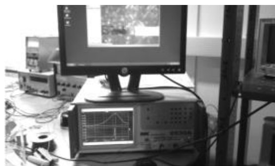
Fig. 5.3: Experimental Setup: the Wayne Kerr Precision Impedance Analyser 6500
