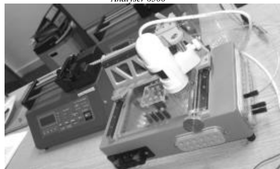
Fig. 5.4: Experimental Setup: The testing base-board, pumps, chip and digital microscope
