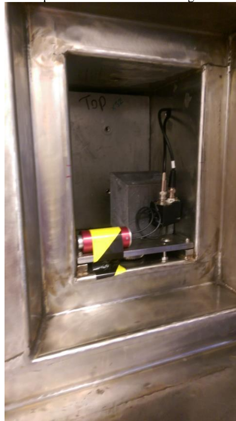
Figure 5. EJ-301 organic liquid scintillator inside the ^{60}\text{Co} irradiator.
