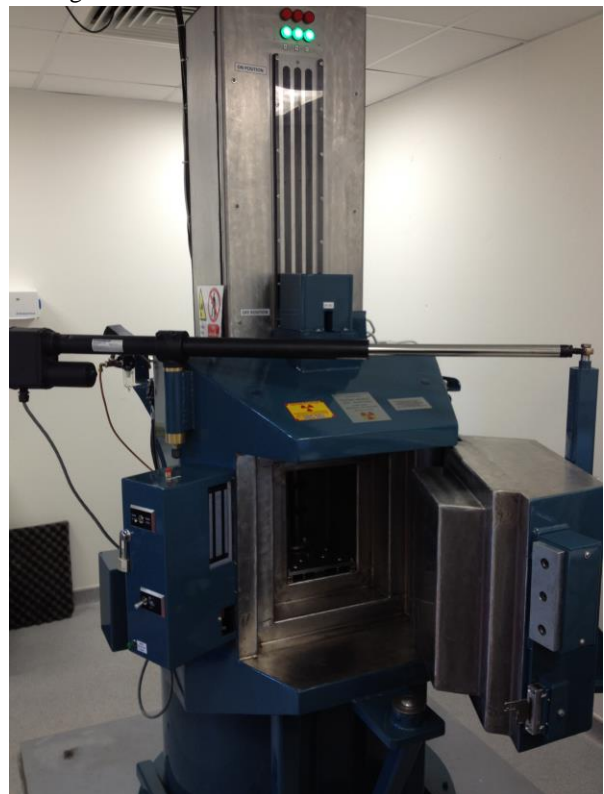
Figure 3. ^{60}\text{Co} gamma irradiator, Foss Therapy Service, Inc. [8]
